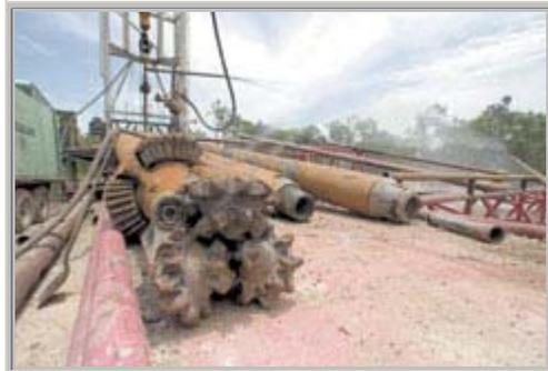
A water well drill bit lies idle Friday after being used to bore a test well at the San Antonio Water System's proposed water well field in western Gonzales County. The testing will help determine whether enough underground water exists at the well field to supply San Antonio with as much as 9.8 billion gallons each year.
